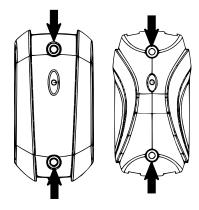
6. Place the plastic lens positioning it properly and securing the top first and then the bottom
