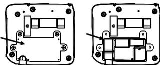
9. Replace and fix the lid and the sealing rubber.
