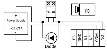
⚠ We recommend the use of an exclusive power supply source to power the Electromechanical Lock.
