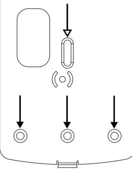
Holes for wall fixing
