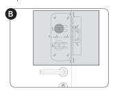
Before drilling the holes, simulate the position of the internal part and the strike and make sure that both are aligned according to the image on the right.
