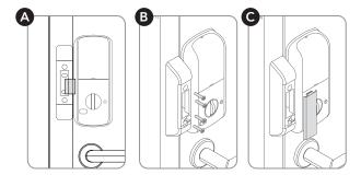
If it is not possible to align the strike and the inner part with or without the spacers (a), make a recess in the door frame to secure the strike using a flat drill and chisel (b).
