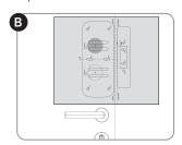
Before drilling the holes, simulate the position of the internal part and the strike and make sure that both are aligned according to the image on the right.
